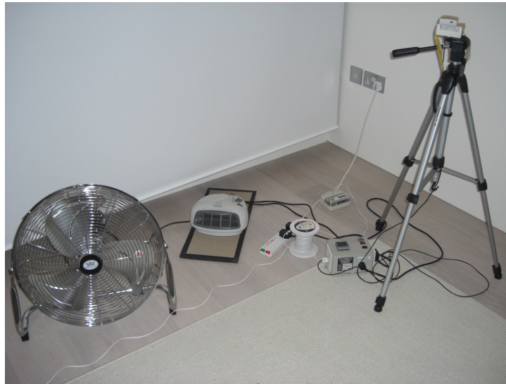
Figure 6: Co-heating zone equipment
