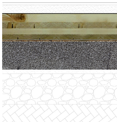
Detail showing the potential to replace with laminated timber and foamglass insulation.
